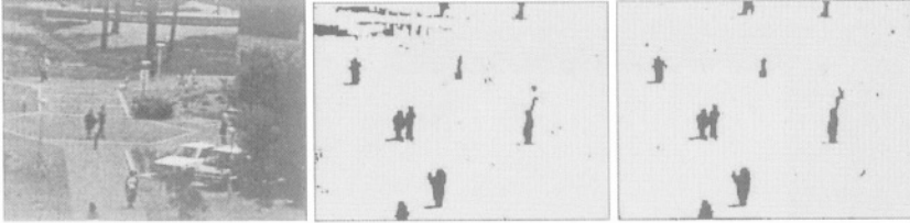
Figure 6.2. Foreground detection under an illumination change: (left) the original frame, (middle) intensity-based foregrounds, and (right) chromaticity-plus-intensity foregrounds.
